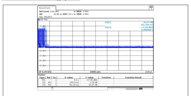
Channel move time = 0.751 250 s Closing time =  $0.000 625 \text{ s} \times 17 = 0.010 625 \text{ s}$
