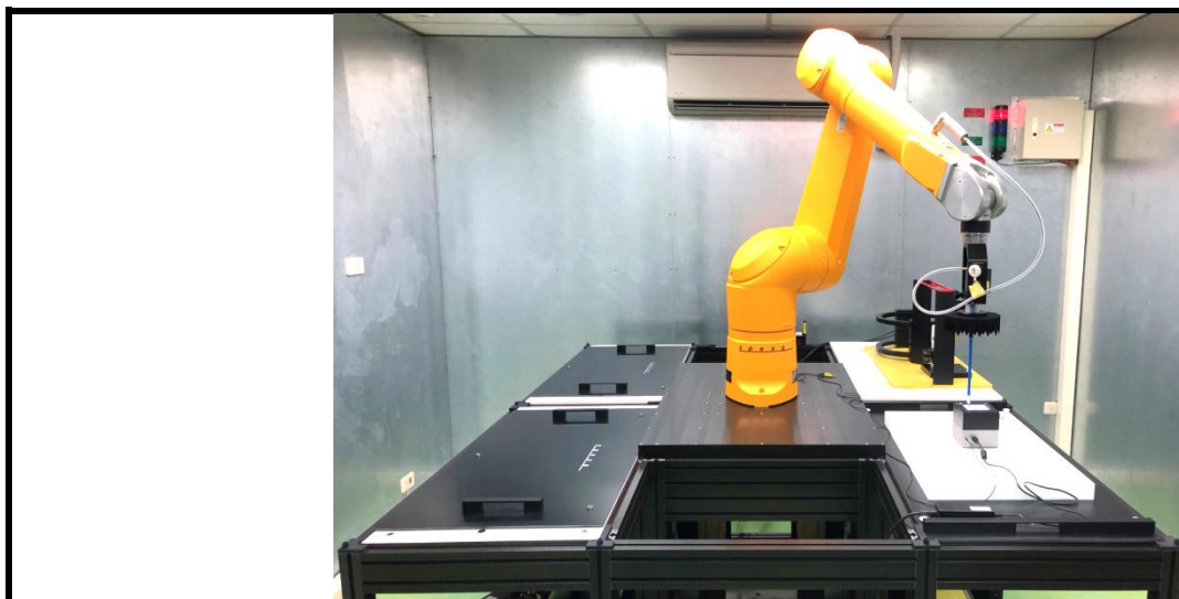
Fig-3.2 SPEAG DASY6 System
