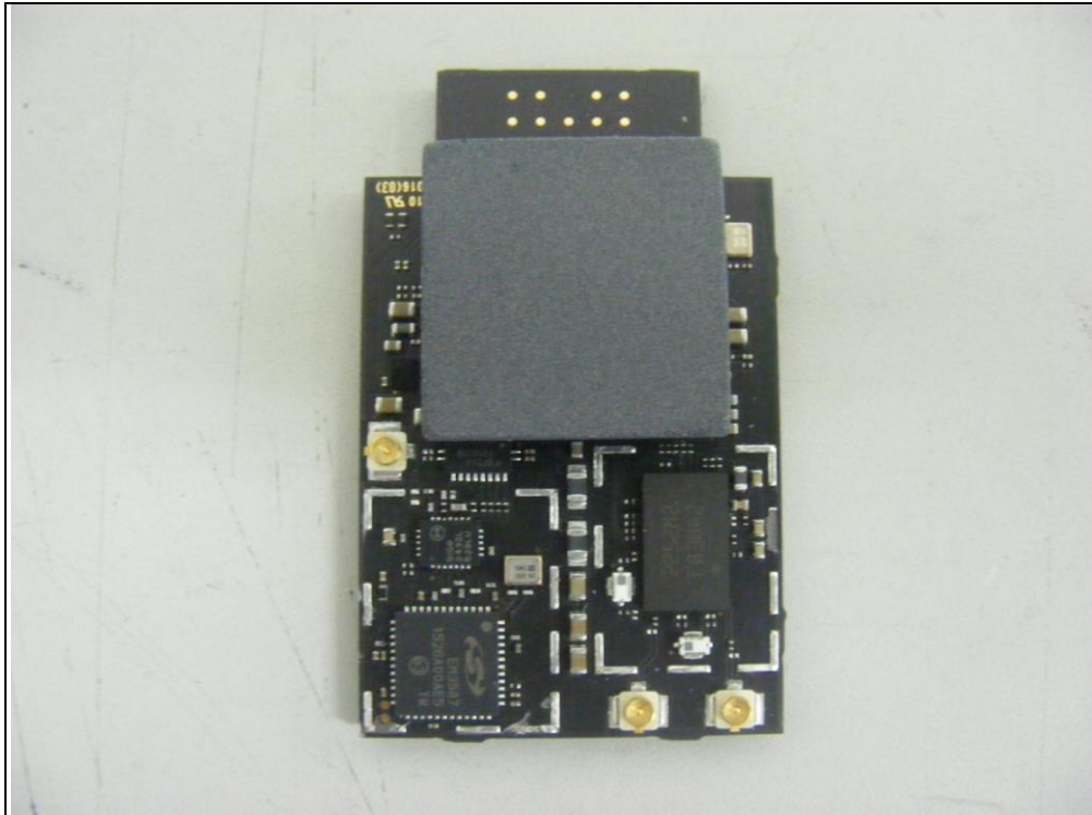
Bottom view of Main PCB
