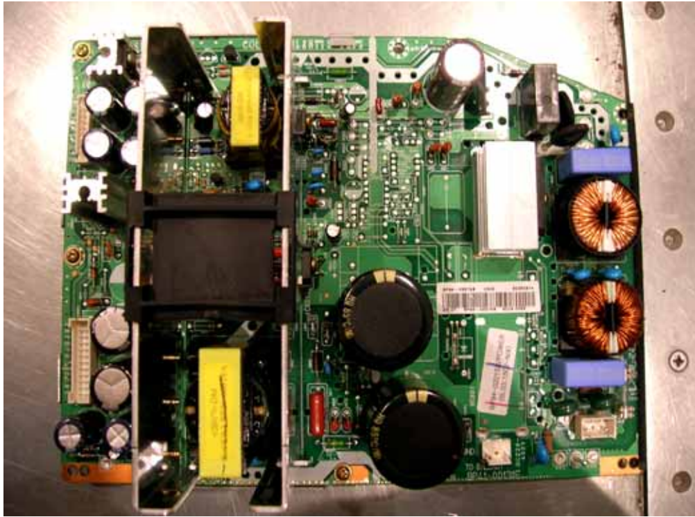
SMPS board top view
