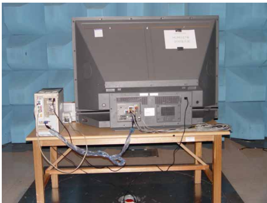
Picture 3. Radiated Emission (rear view)
