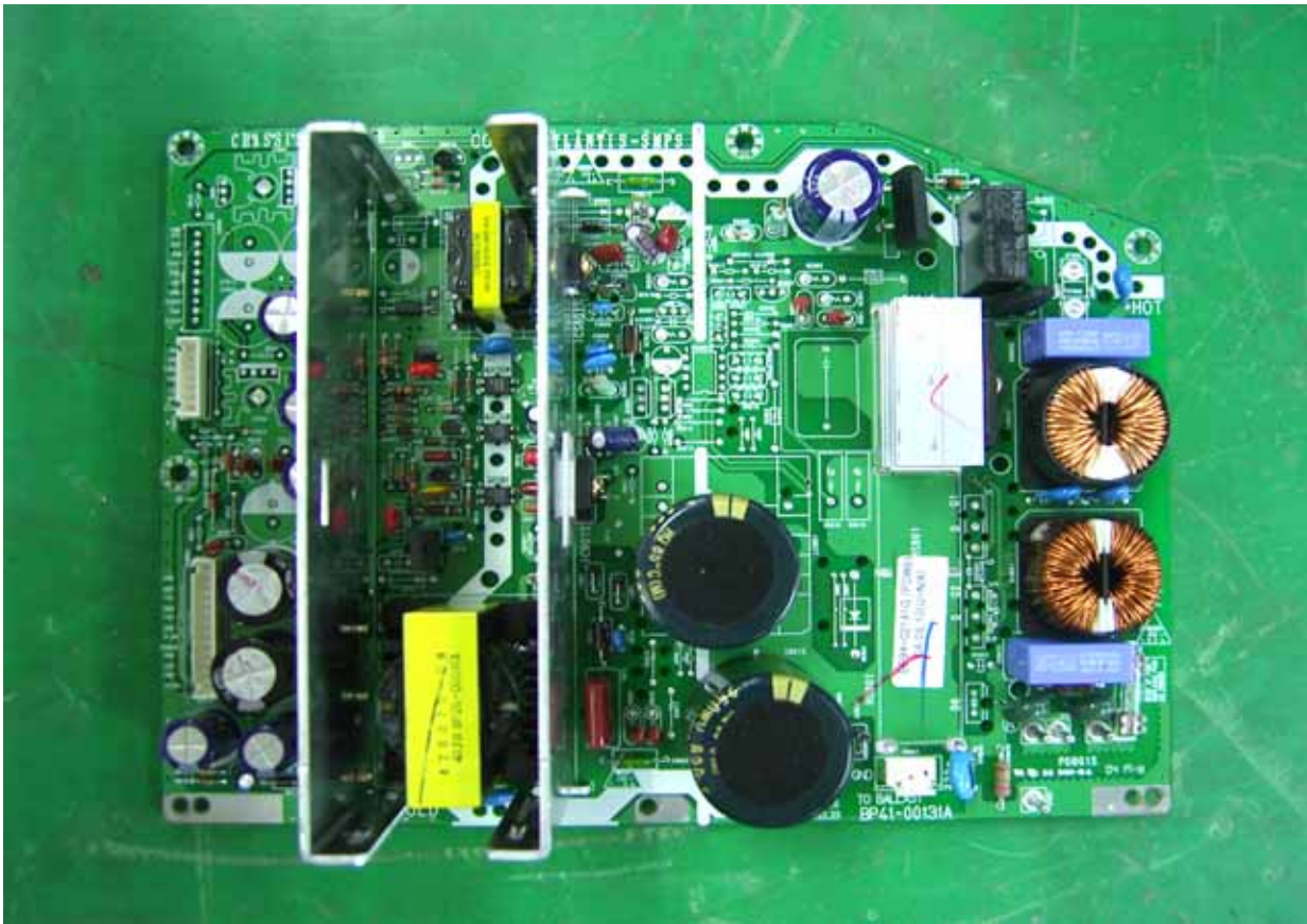
SMPS board top view
