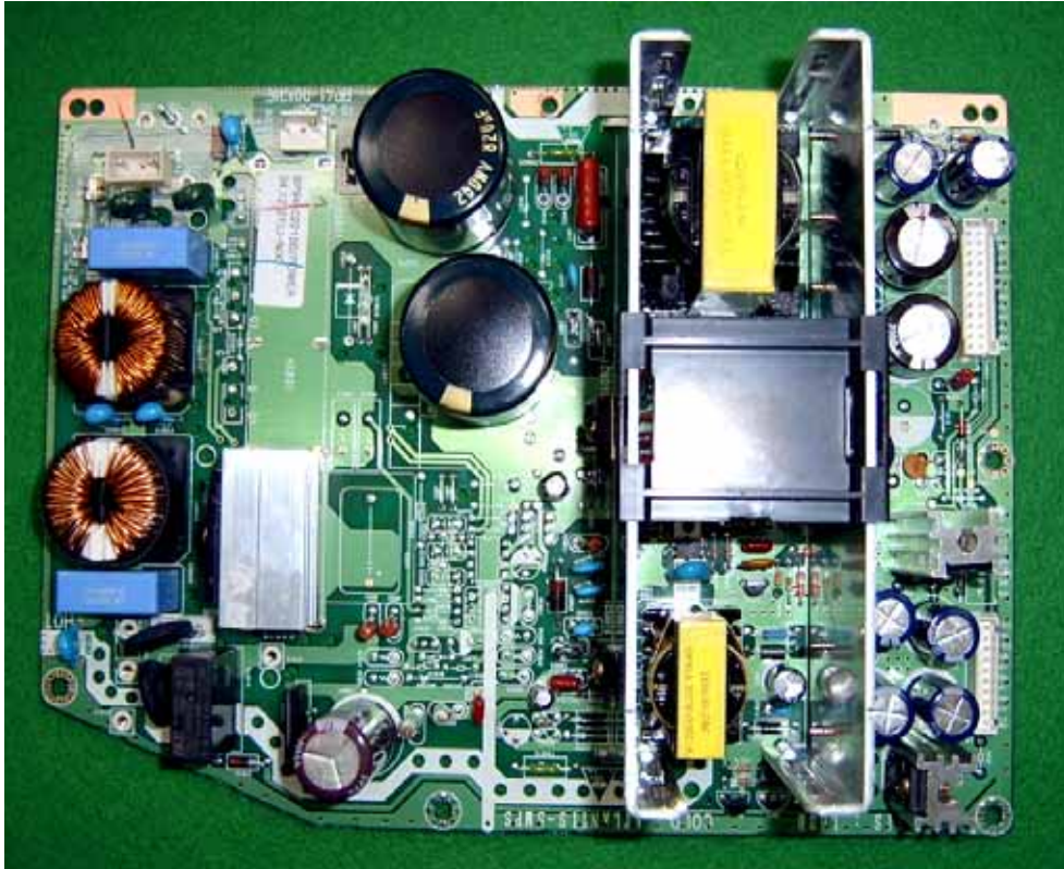
SMPS board top view
