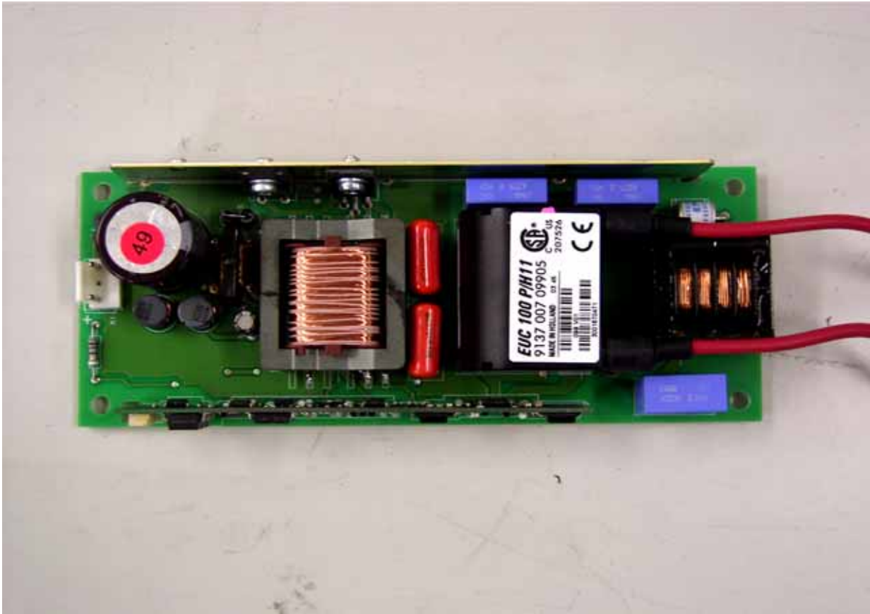
Ballast board top view
