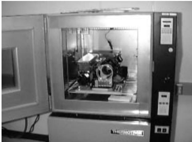
Figure 4. Large-venue XGA 500W engine installed in temperature chamber for temperature testing.
