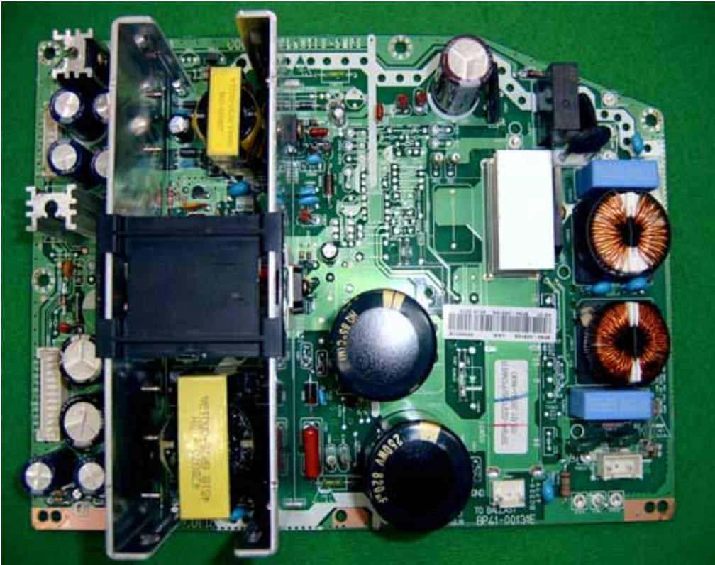
SMPS board top view
