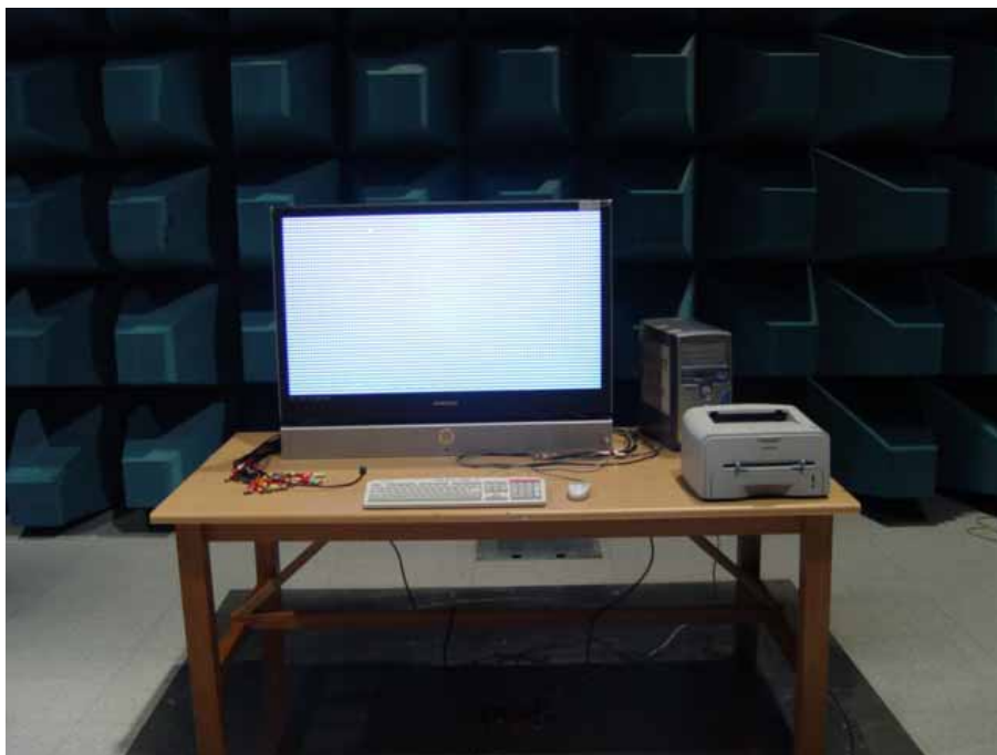
Picture 2. Radiated Emission (front view)
