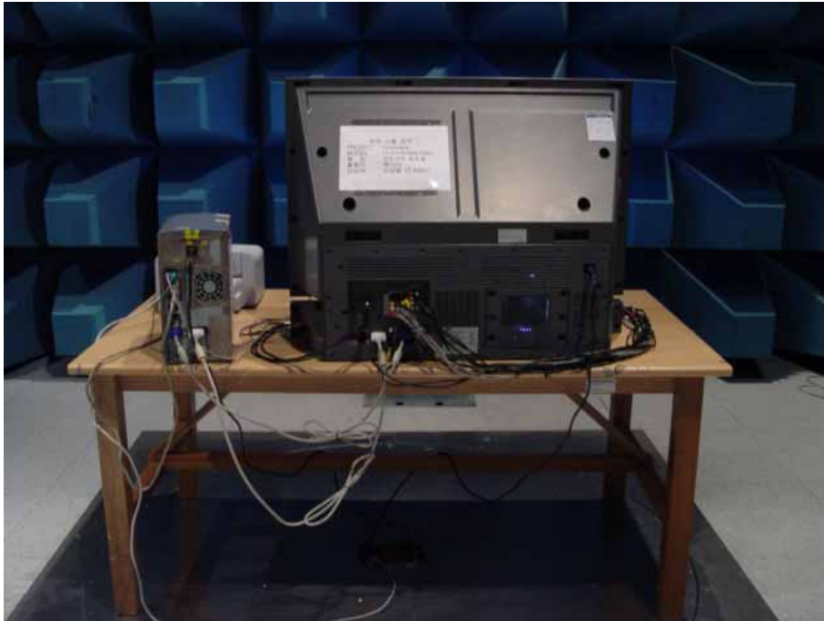
Picture 3. Radiated Emission (rear view)
