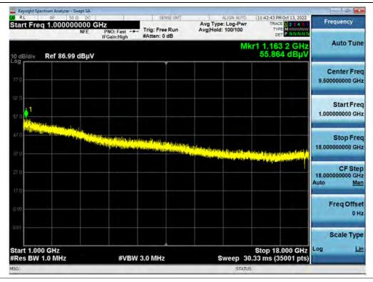
\*In case of 9 kHz to 18 GHz and 40 GHz to 200 GHz, the reading of emissions are attenuated more than 20 dB below the permissible limits or the field strength is too small to be measured so we are attached only the worst case plots.
