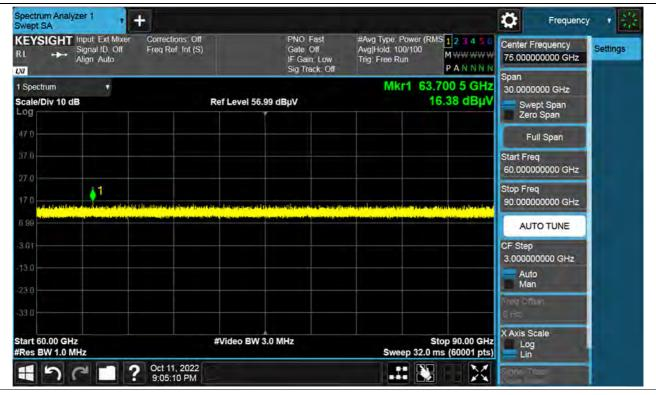
\*In case of 9 kHz to 18 GHz and 40 GHz to 200 GHz, the reading of emissions are attenuated more than 20 dB below the permissible limits or the field strength is too small to be measured so we are attached only the worst case plots.
