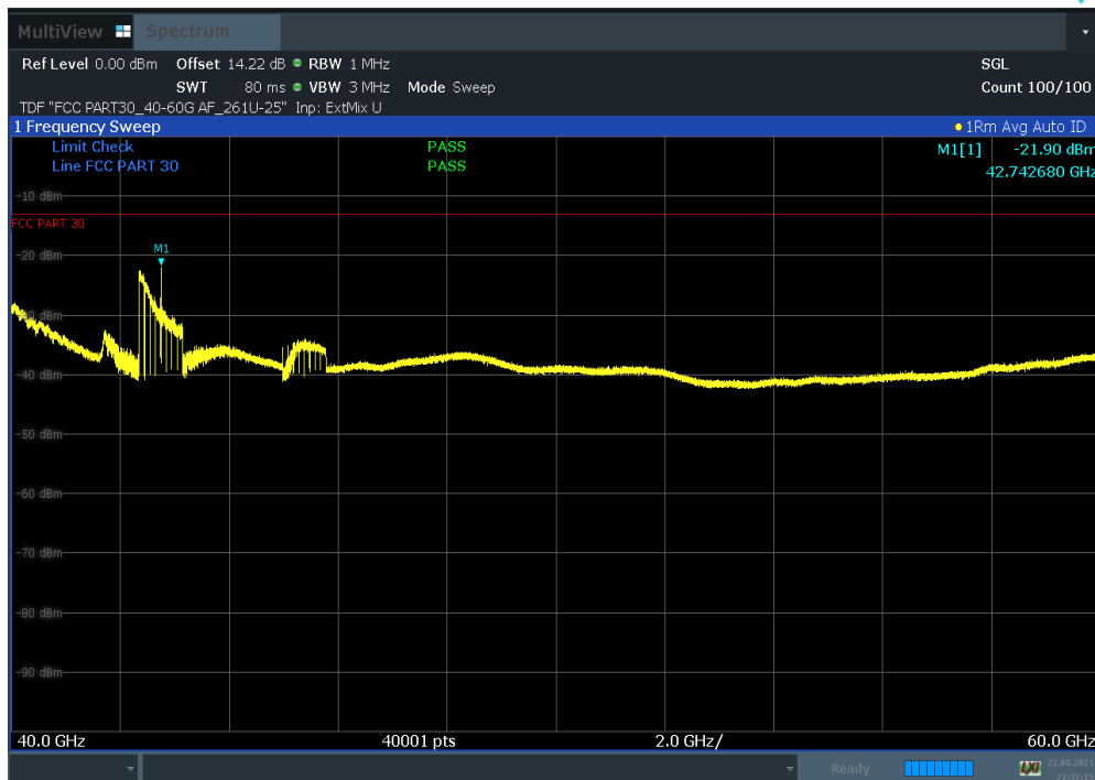
Plot 7-44. Radiated Spurious Plot 40 GHz – 60 GHz (100 MHz 8CC CC BW QPSK Low Channel Pol. V)
