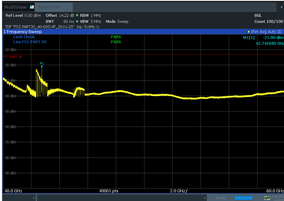
Plot 7-44. Radiated Spurious Plot 40 GHz – 60 GHz (100 MHz 8CC CC BW QPSK Low Channel Pol. H)
