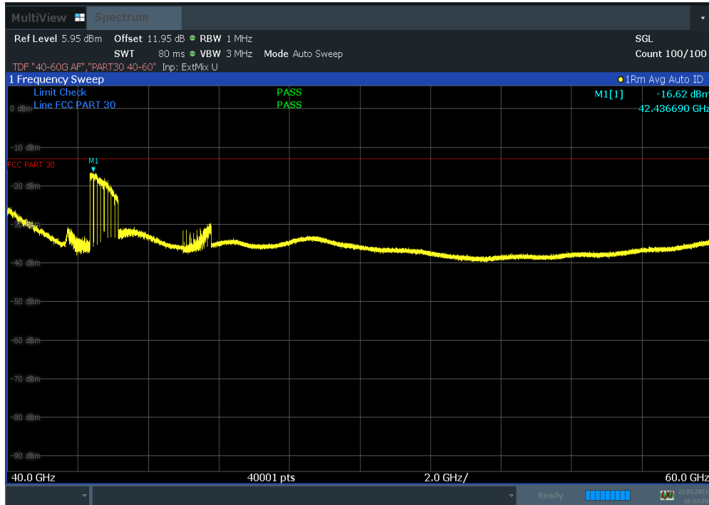
Plot 7-158. Radiated Spurious Plot 40 GHz – 60 GHz (100 MHz 8CC CC BW QPSK Low Channel Pol. V)
