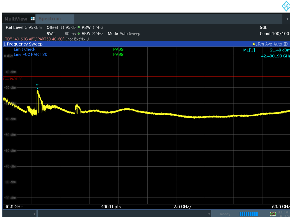
Plot 7-157. Radiated Spurious Plot 40 GHz – 60 GHz (100 MHz 8CC CC BW QPSK Low Channel Pol. H)
