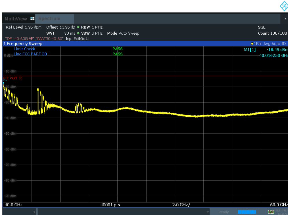
Plot 7-161. Radiated Spurious Plot 40 GHz – 60 GHz (100 MHz BW 8CC NC QPSK Low Channel Pol. H)
