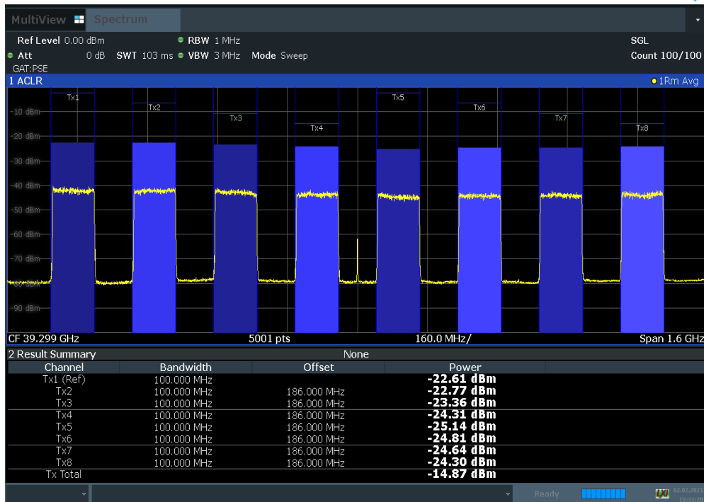
Plot 7-78. Antenna B EIRP Density Plot (100 MHz BW 8CC NC 64QAM High Channel)
