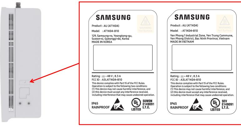
X The label is affixed via suitable adhesive tape for application to painted aluminum chassis permanently.
