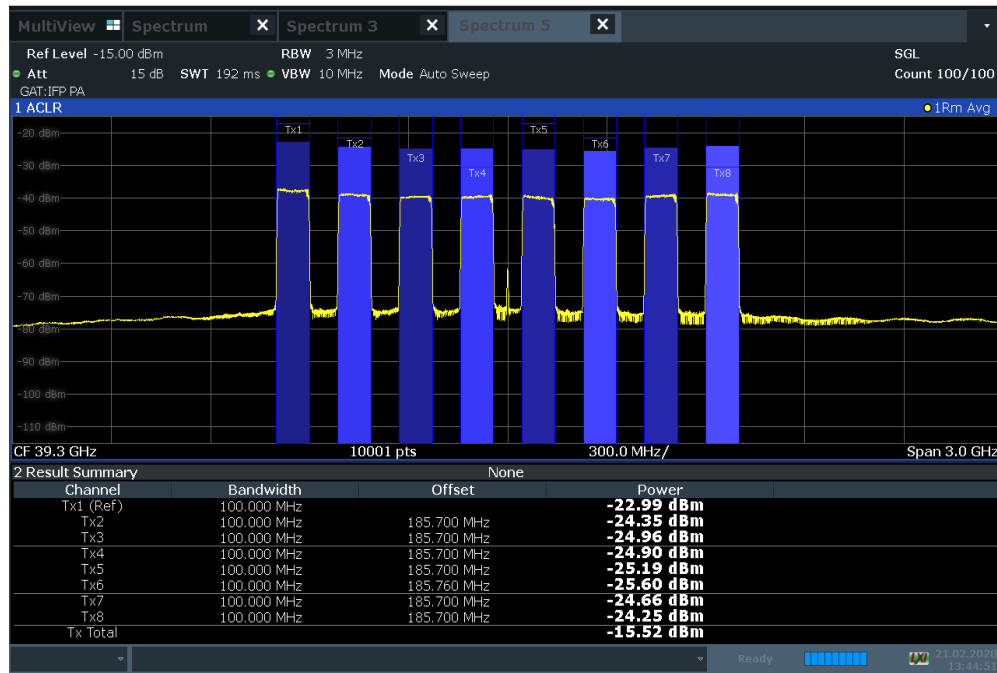
Plot 7-155. Antenna B EIRP Density Plot (100MHz BW 8CC NC 16QAM High Channel)
