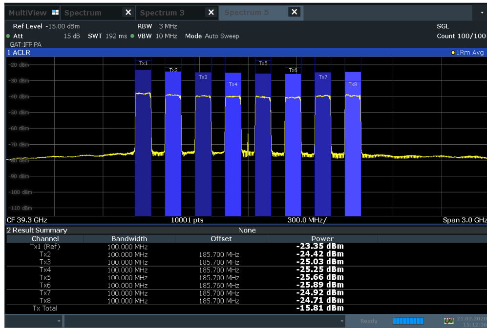
Plot 7-209. Antenna C EIRP Density Plot (100MHz BW 8CC NC 16QAM High Channel)
