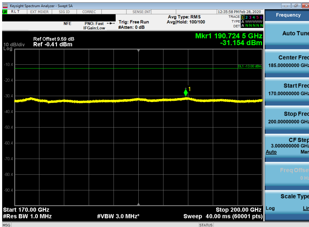
Plot 7-484. Radiated Spurious Plot 170-200 GHz (1CC QPSK High Ch. Ant. Angle 45)
