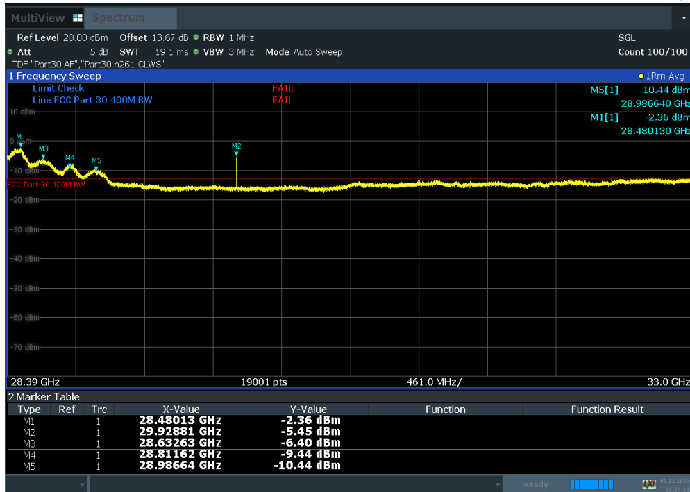
Plot 7-290. Radiated Spurious Plot 28.39 GHz – 33 GHz (50 MHz 2CC + 100 MHz 3CC NC BW QPSK Mid Channel Pol. H) Fin
