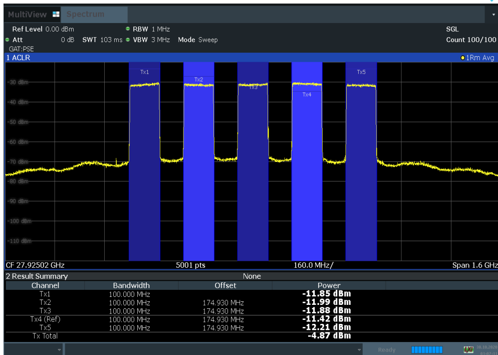
Plot 7-82. Antenna B EIRP Density Plot (100 MHz 5NC BW QPSK Mid Channel)
