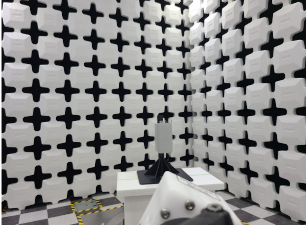
Testing setup for 18 GHz to 40 GHz
