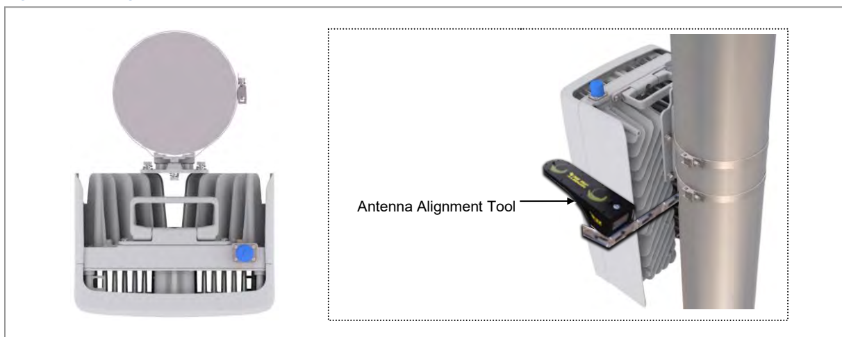
Figure 49. Fixing AU on the Pole (4)
