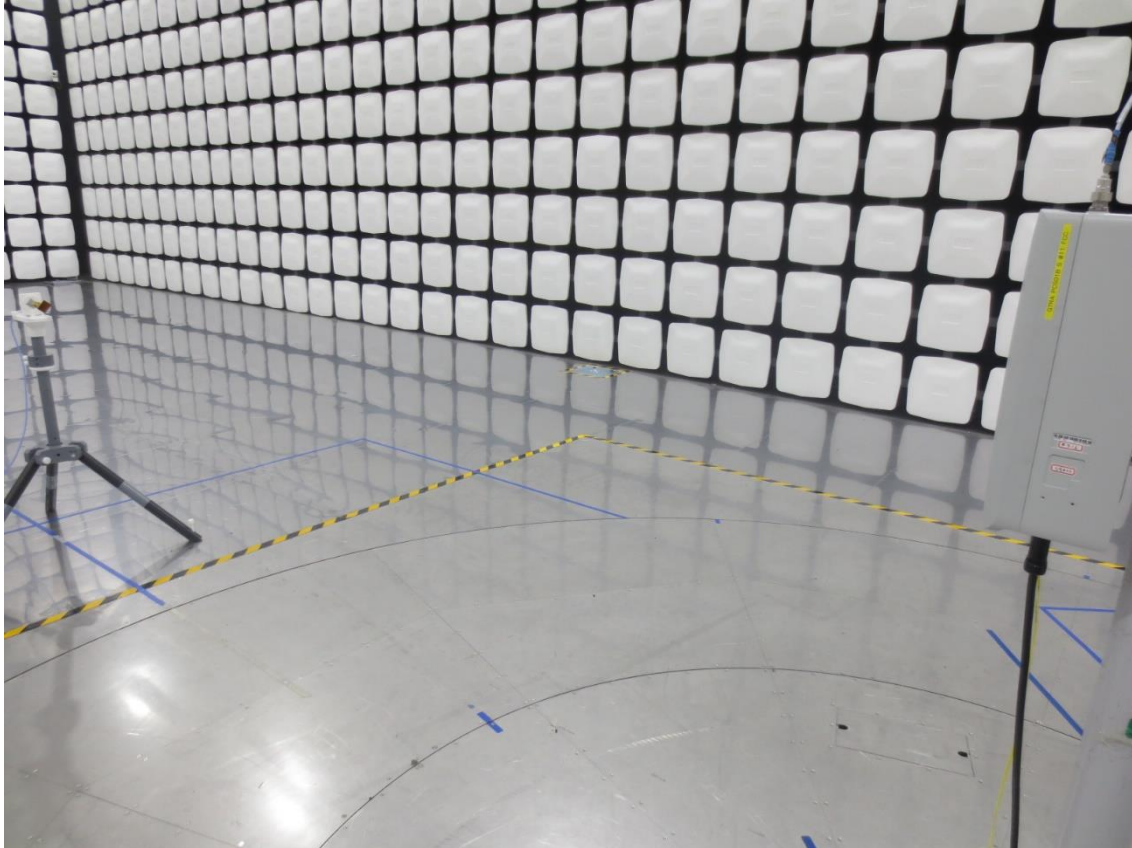
Radiated Test Setup Photo – Spurious (40 GHz ~ 60 GHz, 135°)
