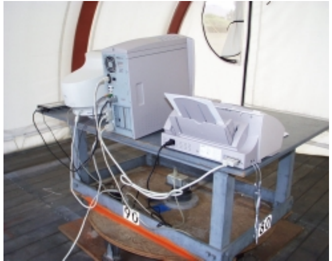
Radiated Emission Setup Photos (Worst Emission Position)
