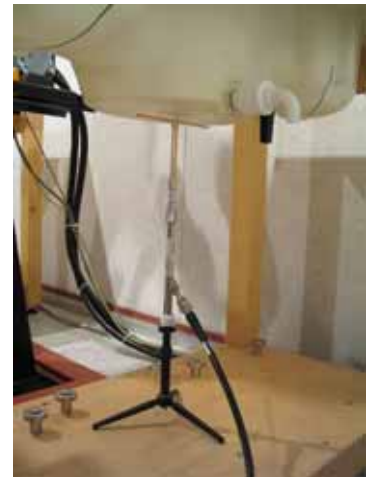
Photo of the dipole Antenna
