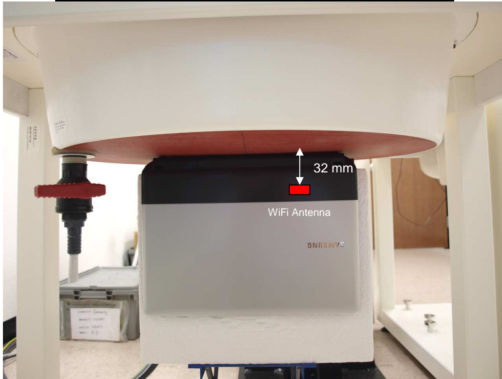
Lap-held, 0 mm from the bottom of the laptop base-to-phantom
