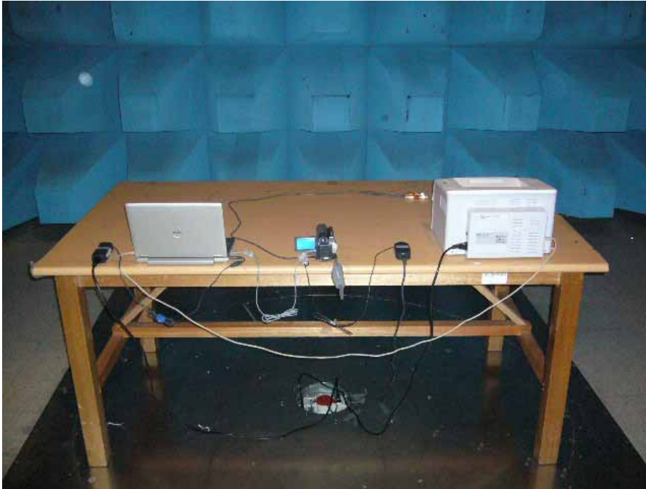
Picture 3. Radiated emission (Rear)
