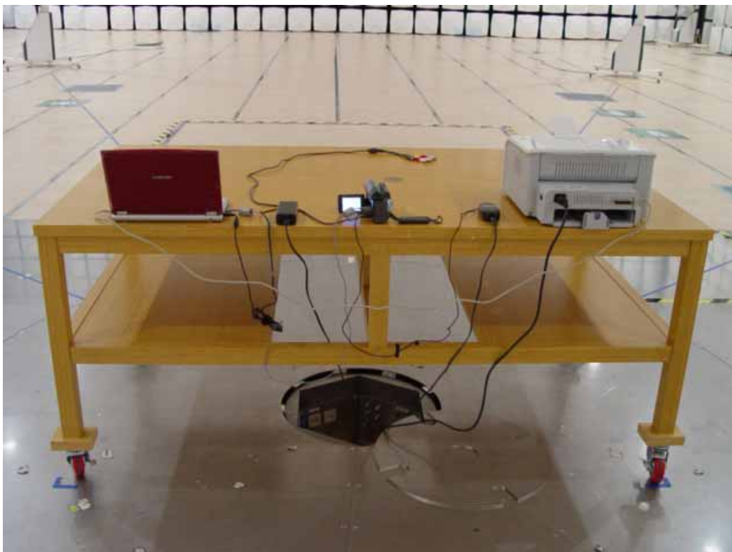
Picture 4. Radiated emission (Rear)
