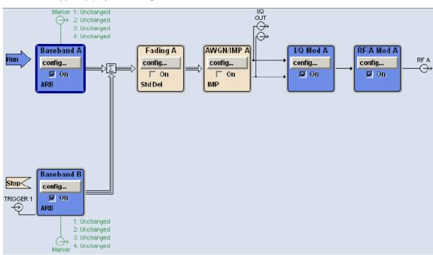
FCC Radar Types (5) System Diagram
