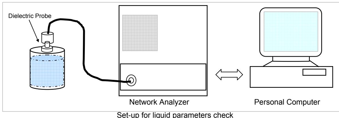
Set-up for liquid parameters check
