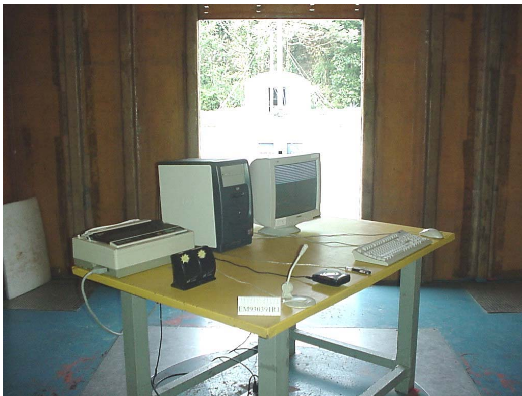
SETUP WITH MAXIMUM DETECTED EMISSION AT VERTICAL POLARIZATION
