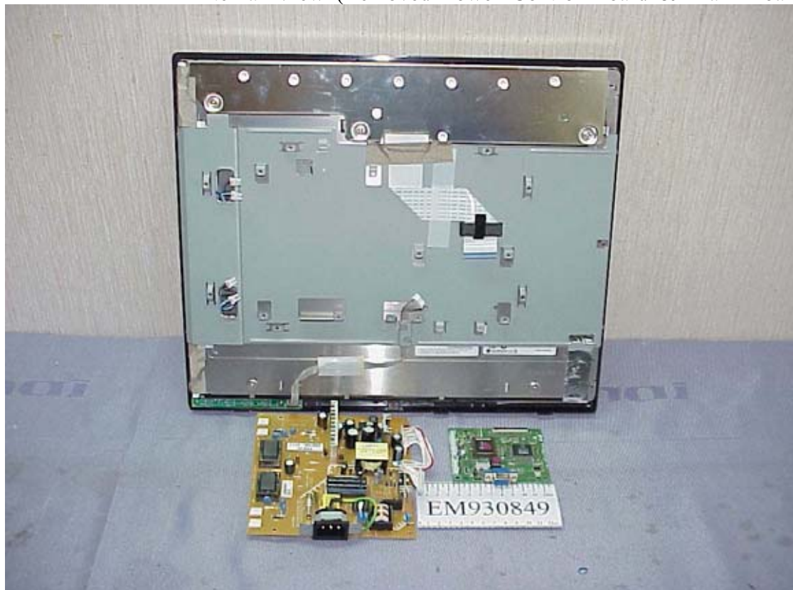
Figure 10 Internal View (Removed Power Control Board & Main Board)
