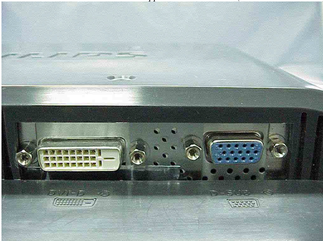
Figure 4 Appearance/Rear View (I/O Ports w/LG.Philips Panel)
