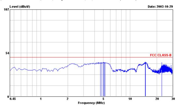
Site : PHILIPS EMI Shielding Room Condition : FCC CLASS-B FCC LCI L2 NEUTRAL
