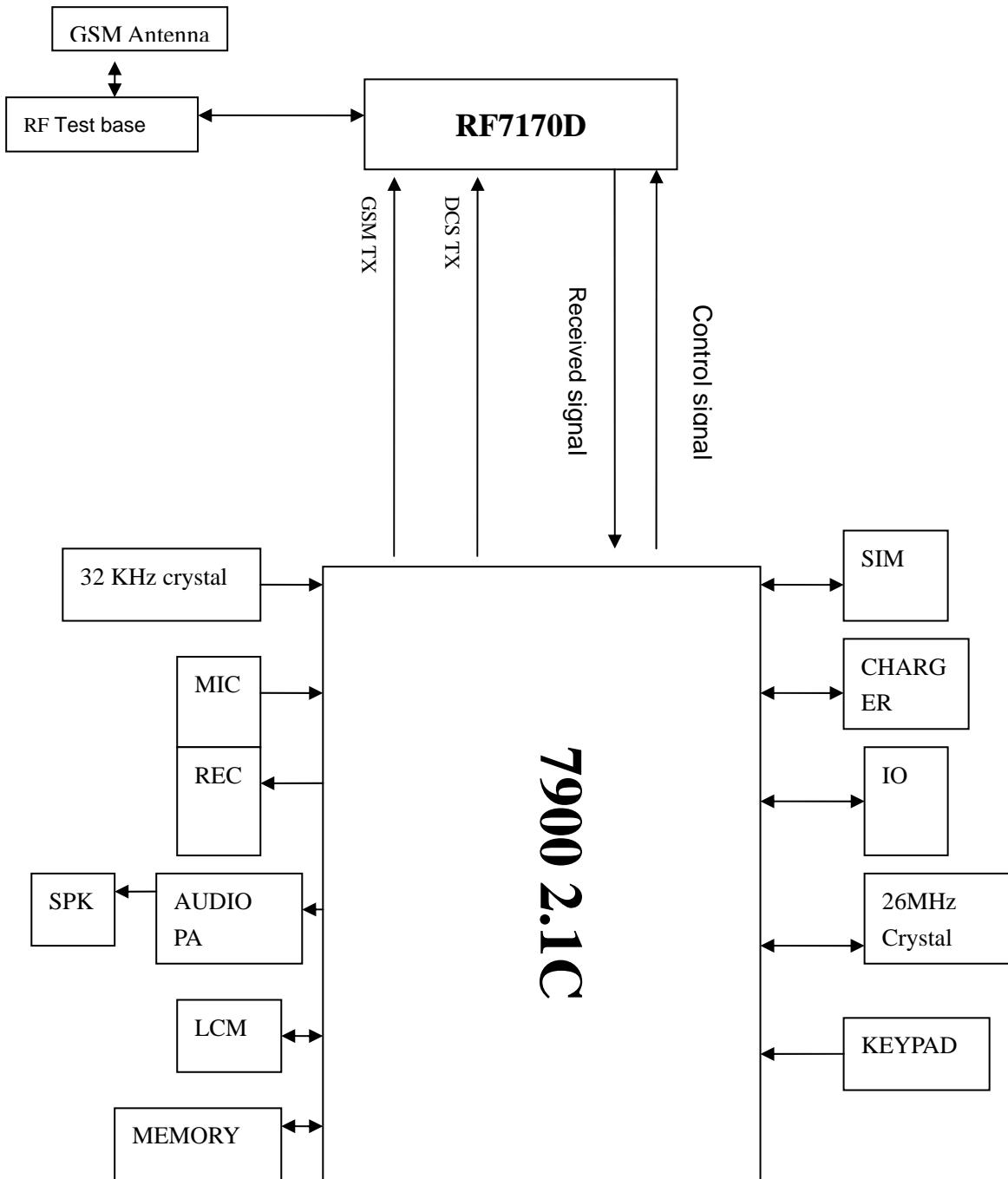
Our project uses the ULC3 platform, and the mainborad is composed of two parts of circuits: BB and RF.
