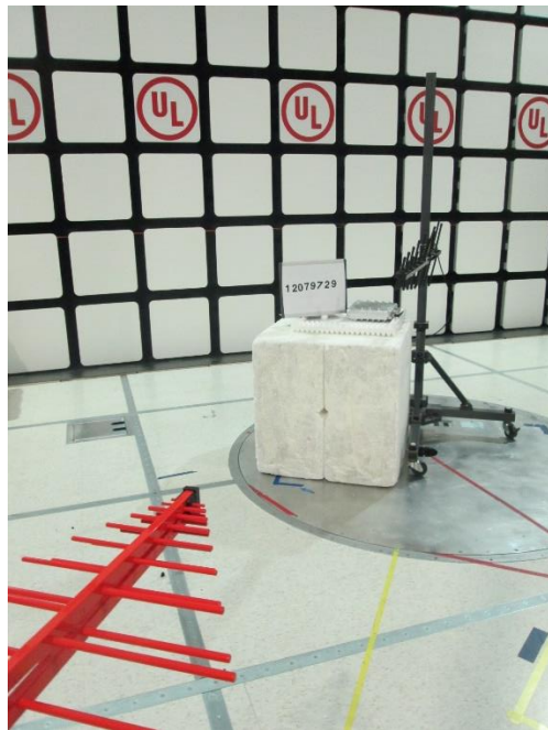
RADIATED BACK UHF LOG PERIODIC ANTENNA
