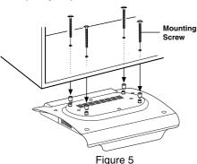
d) Hold each screw head down and push the unit and spacers onto the screws, then hold the unit up until spacers are firmly against the bottom of the cabinet (and fully nested within each other if you are using multiple spacers for each screw).  e) Partially tighten each screw, but do not fully tighten the screws until all of them have been started (see Figure 6).
