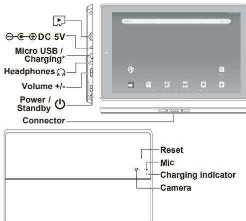
\* Micro USB port for charging at either OFF mode or Standby mode.
