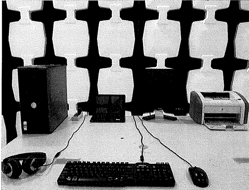
Measurement of Radiated Emission Test Set Up
