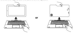
The keyboard connects to the tablet via the Connector. When the connection is successful, the tablet will automatically adjust its settings to use the keyboard.
