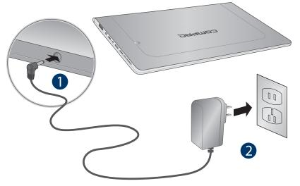
Charging time will vary depending on remaining battery life. Charging from 0%, should take approximately 4-5 hours. Use ONLY the included AC adapter with the small <u>round port</u>. You may not be able to turn on your tablet for at least 20 minutes if the battery was fully drained.
