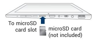
Insert the microSD card into the tablet's microSD slot until it clicks.
