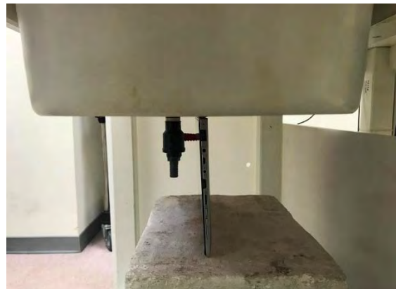
Fig.7 EUT Bottom side to flat phantom
