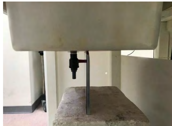
Fig.4 EUT Top side to flat phantom
