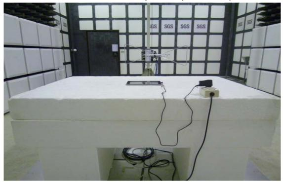
Radiated Emission Set up Photos (Above 1GHz)
