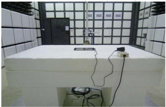
Radiated Emission Set up Photos (Above 1GHz)
