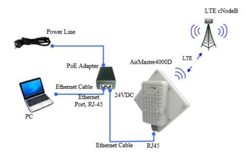
Installing Outdoor Unit (ODU)
