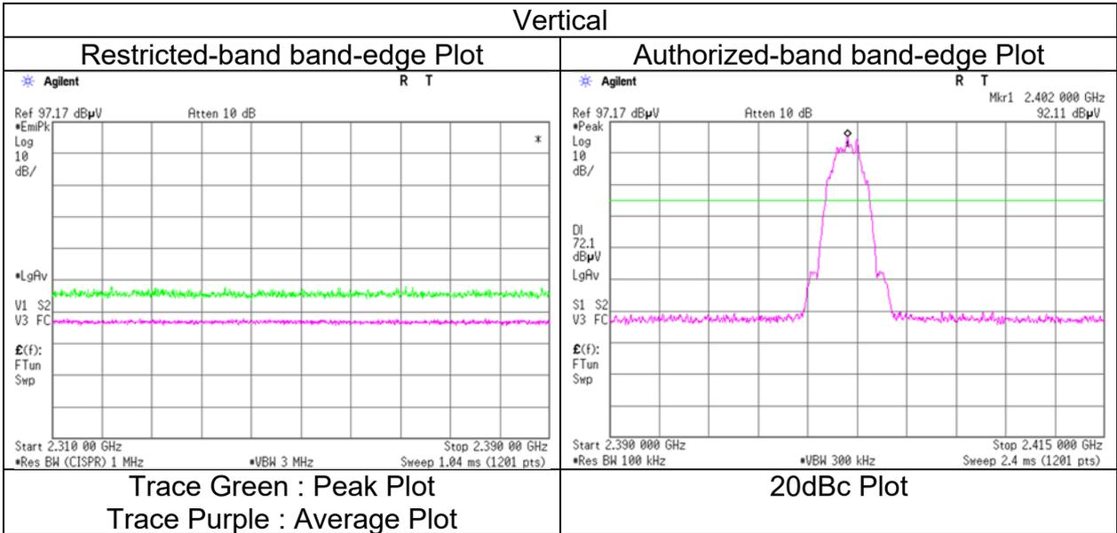
\* The measurement was conducted for a sufficiently long enough time to detect any possible spurious emissions.
