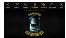
If the car sensor detects an obstacle, the screen automatically changes to the Parking sensor screen. For details, see "About Parking Sensor screen" (page 94).
