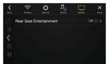
When a Rear monitor equipped with HDMI input is connected to this unit, change this setting to "On." You can output images to the Rear monitor. For details, see "Rear Seat Entertainment Function" (page 19).
