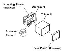
$st^{l}$  If the installed mounting sleeve is loose in the dashboard, the pressure plates may be bent slightly to remedy the problem.
