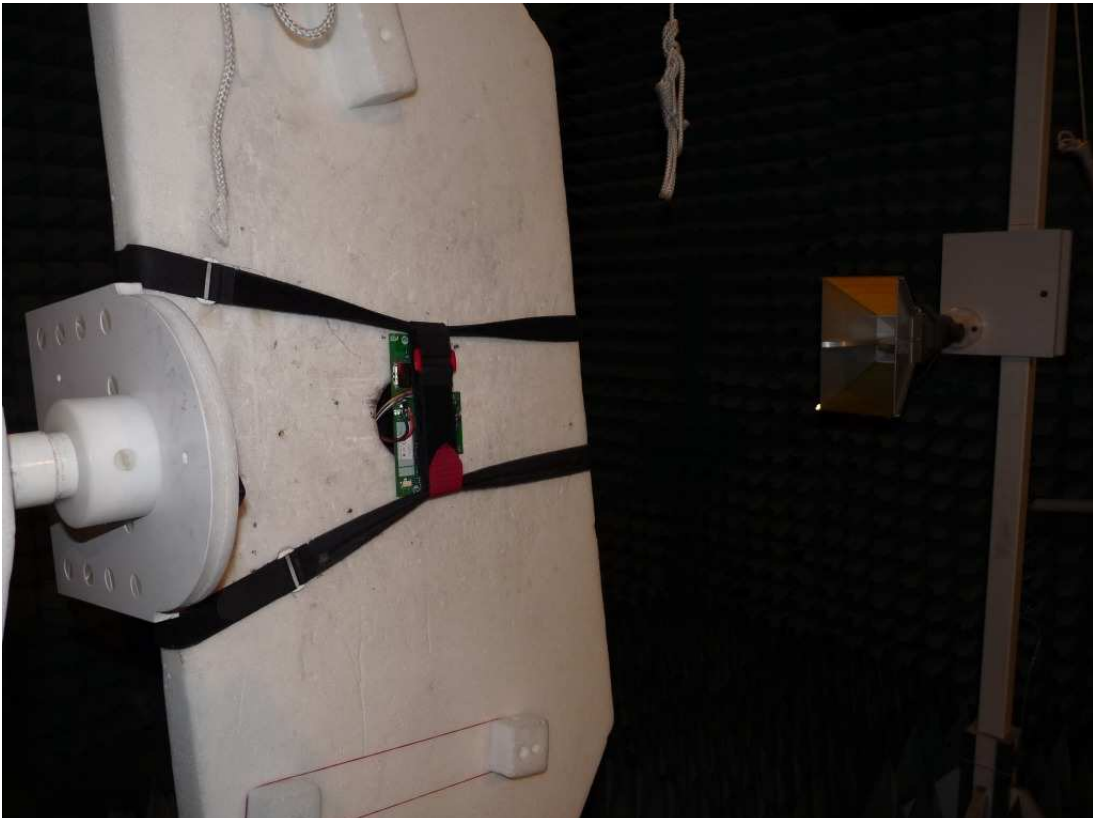
Photo 4: Test setup for radiated measurements (above 1 GHz)
