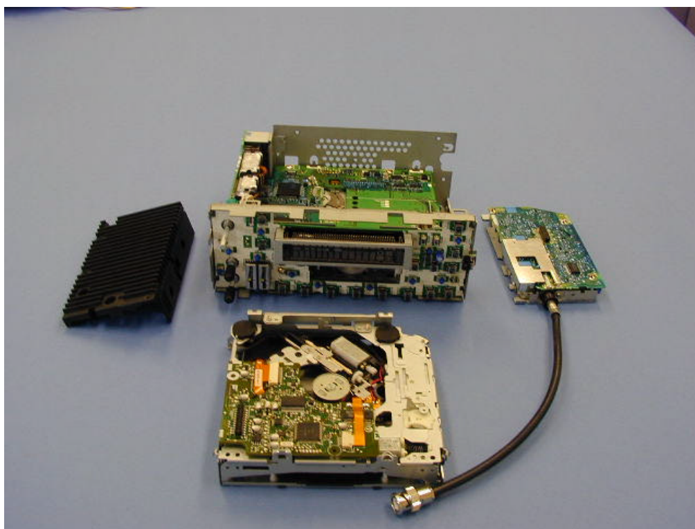
CD Unit & Tuner Module removed
